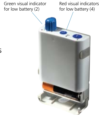
Figure 10: Changing the battery
