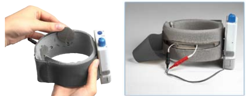
Figures 11 and 12: Changing the electrodes (inside and outside views)
