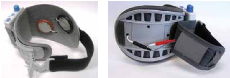
Figures 9 and 10: Changing the electrodes (inside and outside views)
